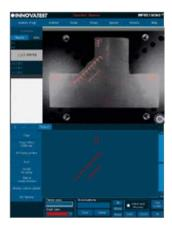
A special application for testing and reporting on the hardness tracking of welds according to ISO 9015 standards. Combined with automatic edge detection this software tool improves measuring welds according to standards efficiently.
